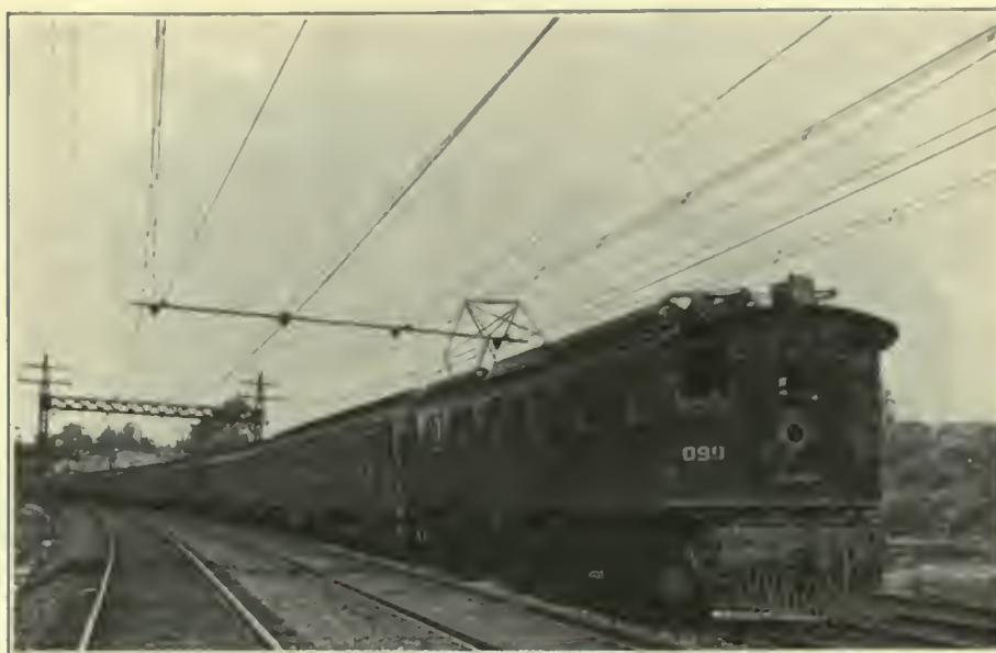
FIG. 538. ELECTRIC LOCOMOTIVES. Locomotive and Train for 11,000-Volt Single-Phase Overhead Contact Operation, New York, New Haven & Hartford Railroad.
